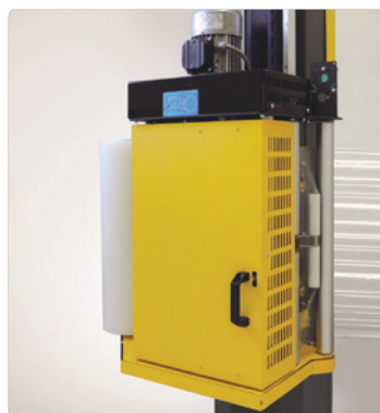
LP - Powered pre-stretch 240% (150%-200% - kit available as option)
